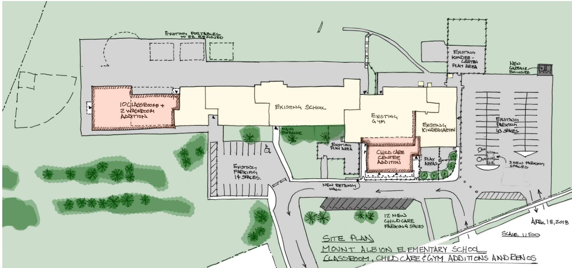
Architect illustration of proposed site plan including the new additions.
